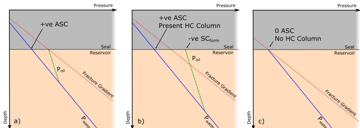
Figure 1. Schematic pressure-depth plot indicating the ‘conventional’ route for mode I failure (a) and the new approach (b & c) suggested by Swarbrick et al. (2010)
